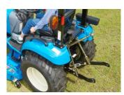
Durable And Adjustable Three Point Provides 1,433 lbs. Of Lift Capacity
