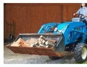
High Capacity Front Loader Features 1,276 Lbs. Of Lift Capacity At Pivot Pins
