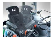
**Premium Seat** The Air Suspension Seat With 10 Degree Swivel For Added Comfort
