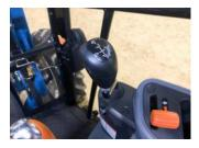
Integrated Loader Joystick Enables Precise Control Of The Front-Loader
