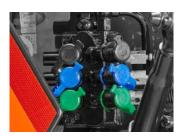
Available With Three Rear Remotes (Cab Only) Provides Added Flexibility For Attachments And **Implements**
