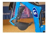
*Optional Thumb Configuration Backhoe* Provides Added Functionality To The Heavy-Duty Backhoe
