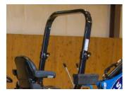
*Standard Foldable ROPS* Enables Easy Adjustment For Clearance
